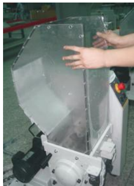
Picture 3-9: Installation of Feed Box, Feed Port and Storage Bin 1
