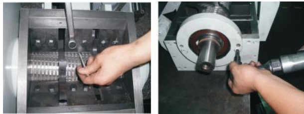
Picture 6-3: Dismantle Rotate Blades
