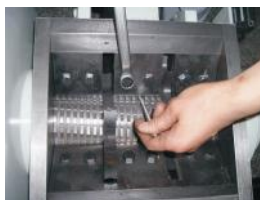
Picture 3-6: Installation of Teeth Cutter and Fixed Blade
