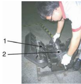
Picture 3-4: Installation of Bearing and Cutter Shaft 2
