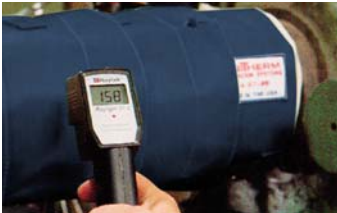
A comparison of manual surface temperatures with and without a UNI-VEST™ shows a difference of 471° F.
