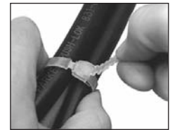
3. To Lock: Pull end up to lock in place. To Release: Pull end of strap out and then down.
