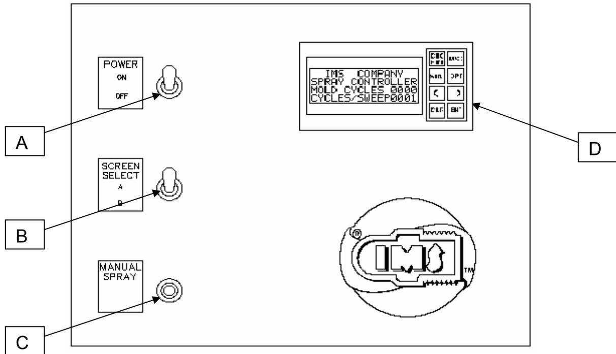
1. Once all connections have been made, the controller can be switched on using the **POWER SWITCH (A)** on the front panel.
